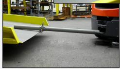
The "Tow Clamp" connects between the ramp pocket and the tow hitch of your fork truck and permits easy transportation of the lift over longer distances.
