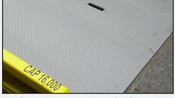
A 60" transition at grade and 30" transition at dock height is constructed of high strength diamond tread plate beveled and recessed for smooth transition onto and off the yard ramp.
